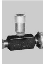
A flow control valve is provided to adjust the machine RPM. Adjusting the speed can greatly reduce blade chatter for a cleaner, more accurate machined surface. Turning the knob clockwise slows the cutting blade speed.
