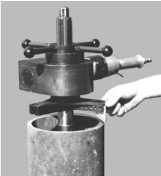
A variety of standard tooling is available to perform I.D. and O.D. beveling, squaring and J-beveling. Custom designs are also available to match your specific requirements. The blades are "SM" type, resharpenable. The same tooling is used for both models.
