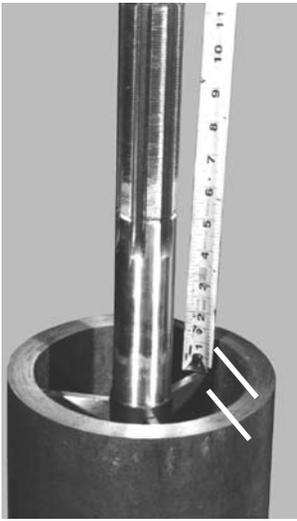
For O.D. machining, the center shaft and wedge assembly should be positioned where the end of the wedge plate is between 1" and 2" (25 mm and 51 mm) from the edge of the pipe to be machined. **For I.D. beveling, the wedge plates must be at least 1" (25 mm) deeper than the tip of the blade at completion of the cut.**
